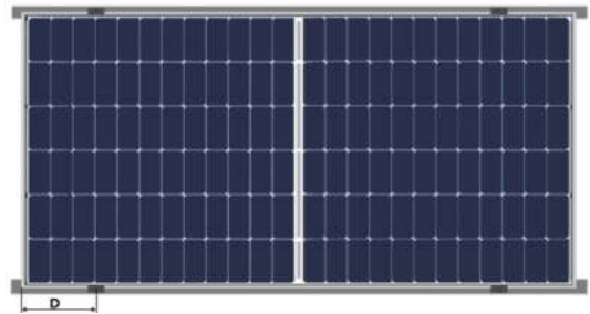
Installation of framed module with fixtures on long sides (beam parallel to long sides) (clamp length \geq 40\text{mm} )
